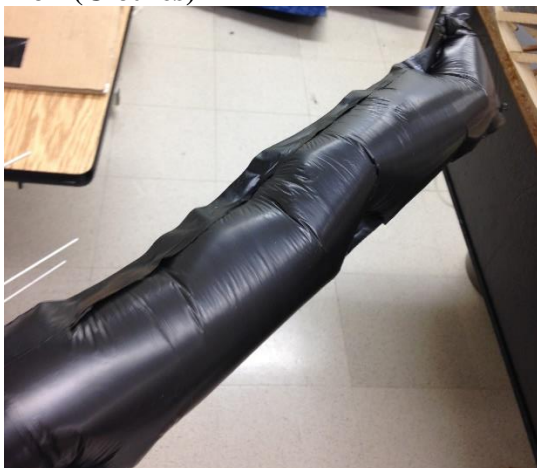
Small balloon made from clothing iron using the folded side method with aluminum. At first it held up, but under greater pressure failed.
