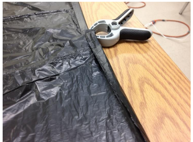
Folding of edges of plastic bag. Increases bond of sheets, but decrease volume of balloon
