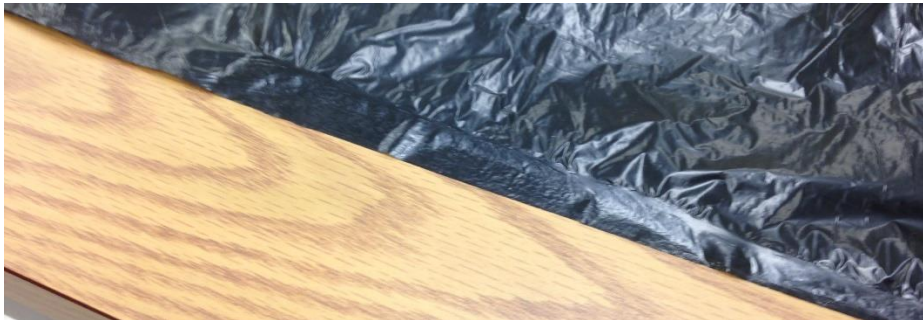
The strongest bond resulting from the Flat Iron, Aluminum foil method. Not the increase in reflection, as compared to the rest of the bag, where the seam is.
